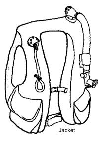
overpressure vent valve and inflator are working properly. If your BC is equipped with a carbon-dioxide inflator, remove the CO2 cartridge and replace it with a spent cartridge or regulator port plug to prevent accidental inflation, which may pin you against the ceiling.
