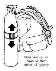
Weights. In addition to lowering your center of buoyancy by modifying the BC, you can also raise your center of gravity by moving your lead weight upward. When cavern diving you do not want to ditch your weights, otherwise the uncontrolled resulting positive buoyancy may pin you against the Thus, a quick-release ceiling. weight belt is not needed and you can attach your lead almost anywhere. To raise your center of gravity, attach your lead weights to your
