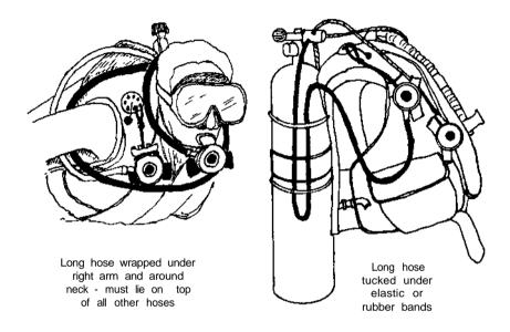
from the regulator you are passing off and it has a long hose, the excess hose is generally stored in one of two ways. It is either held in place by an elastic strap attached to the tank valve or it is routed along the side of the tank and secured with an elastic band; the second stage is then routed under the right arm and secured on the shoulder with an octopus retaining strap.
